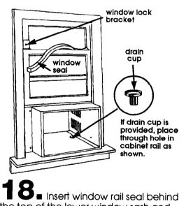
the top of the lower window rail seal berning against the glass of the upper window. Place window-lock bracket on top of lower window and against upper window sash. Use a 2.4 mm (3/32") drill bit to drill a starter hole through the hole in the bracket. Attach window-lock bracket with wood screw. Seal small openings around window with gum-
